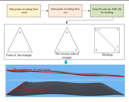
Fig. 8 Construction method for the coal seam cutting floor based on a mesh grid
