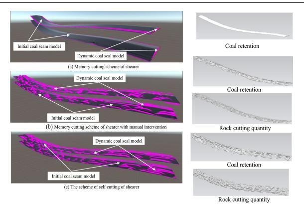
Fig. 15 3D schematic of the fully mechanized mining equipment workspace with three cutting schemes
