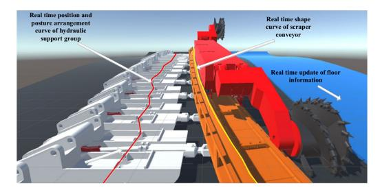
Fig. 14 Straightness information extraction of the scraper conveyor and hydraulic support groups
