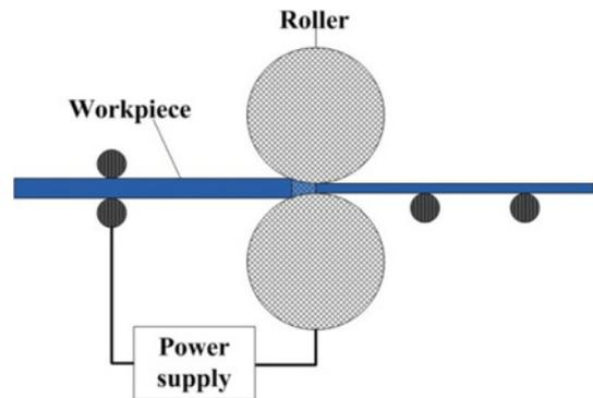
Fig. 8 A schematic of the EA rolling process (modified and redrawn from Ref. 75)
