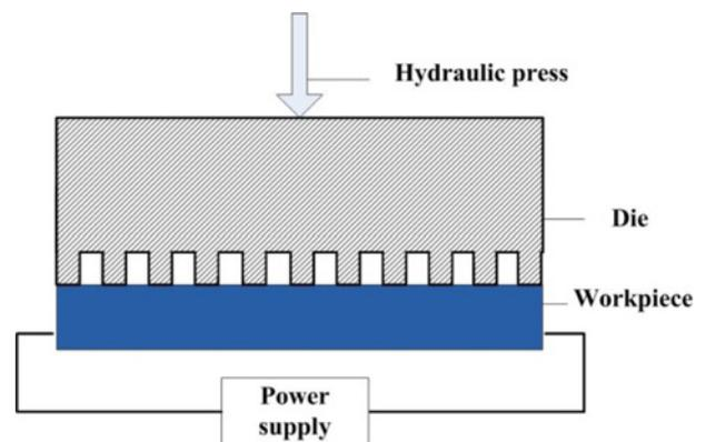
Fig. 11 A schematic of the EA embossing process (modified and redrawn from Ref. 84)
