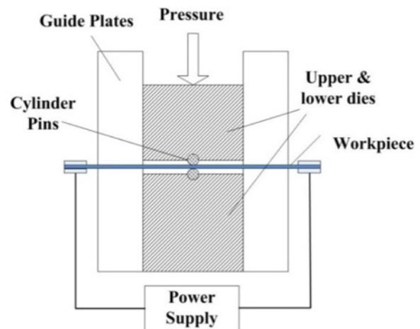
Fig. 16 A schematic of the EA pressure welding process (modified and redrawn from Ref. 92)
