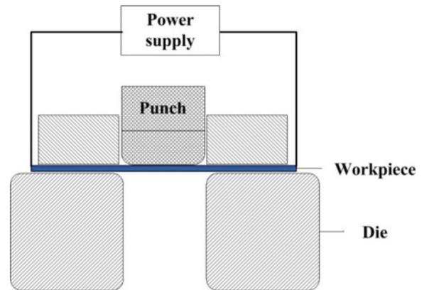
Fig. 10 A schematic of the EA deep drawing process (modified and redrawn from Ref. 83)
