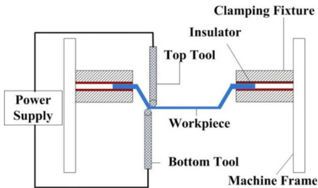
Fig. 14 A schematic of the EA incremental forming process (modified and redrawn from Ref. 88)
