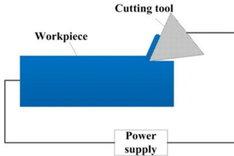
Fig. 17 A simplified schematic of the EA cutting process (modified and redrawn from Ref. 93)
