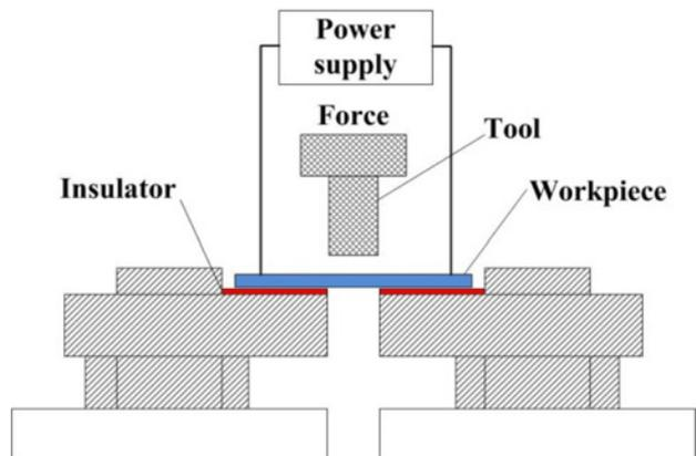
Fig. 12 A schematic of the EA blanking and RH blanking processes (modified and redrawn from Ref. 85)
