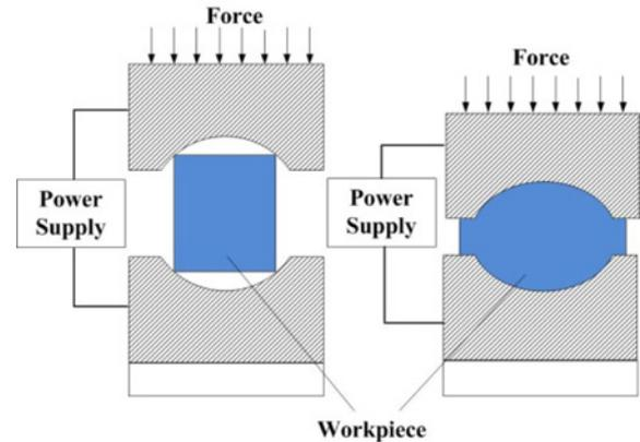
Fig. 7 A schematic of the EA forging process (modified and redrawn from Ref. 70)
