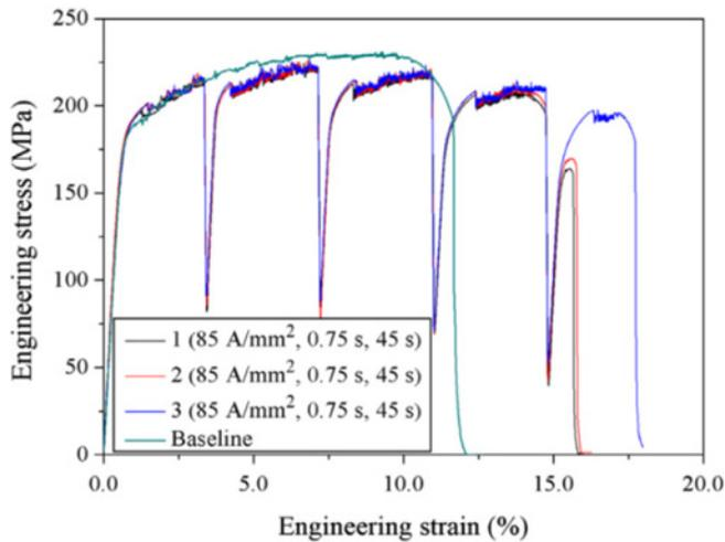
Fig. 2 Experiment results of 5052-H32 aluminum alloys under a pulsed electric current<sup>18</sup>
