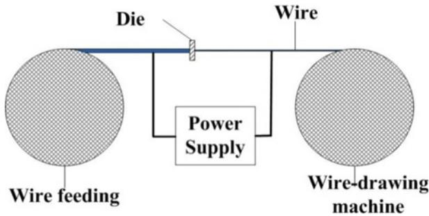
Fig. 9 A schematic of the EA drawing process (modified and redrawn from Ref. 77)
