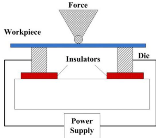
Fig. 4 A schematic of the experimental setup for the EA bending test (modified and redrawn from Ref. 40)
