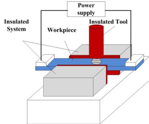
Fig. 15 A schematic of the experiment setup of the EAFSW process (modified and redrawn from Ref. 91)
