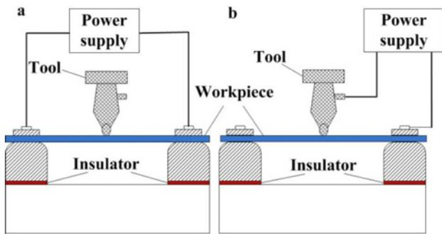
Fig. 13 A schematic of EA stretch forming processes; (a) Across the workpiece (b) Through the tool to the workpiece (modified and redrawn from Ref. 86)
