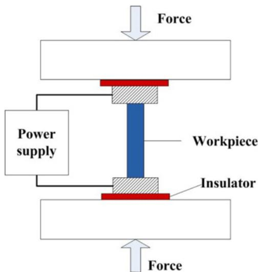
Fig. 3 A schematic of the experimental setup for the EA compression test (modified and redrawn from Ref. 63)
