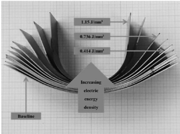
Fig. 5 Springback reduction of advanced high-strength steels with various current densities<sup>67</sup>
