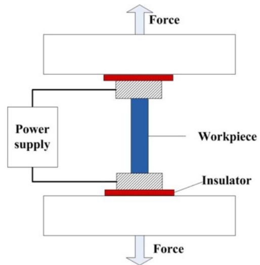
Fig. 1 A schematic of the experimental setup for electrically-assisted tensile testing (modified and redrawn from Ref. 14)
