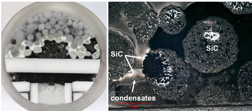
Fig. 6—Sample from experiment no 9. From the right light microscope images of the pellets, condensates and SiC.
