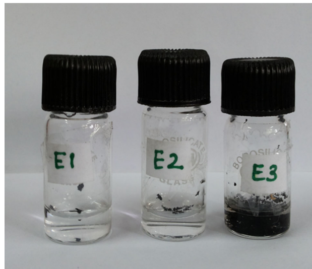
Fig. 13 Photograph with samples E1, E2 and E3 dispersed in water and ultrasonicated for 1 min, showing hydrophilicity of sample E3
