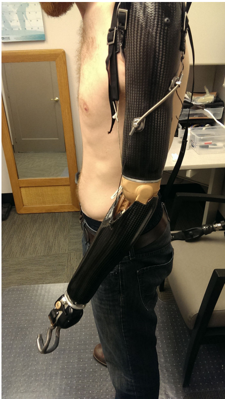
Fig. 4 Transhumeral hybrid system with electronic terminal device (ETD)
