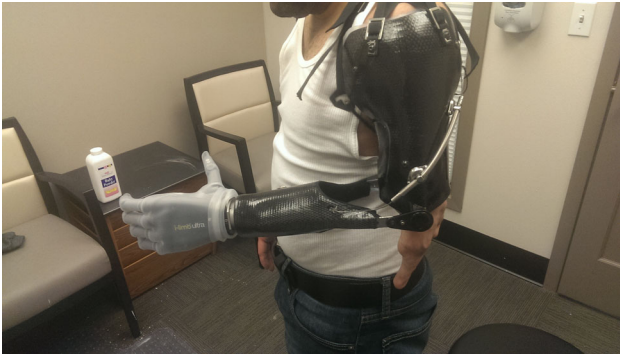
Fig. 2 Congenital above elbow hybrid system with conforming grasp hand
