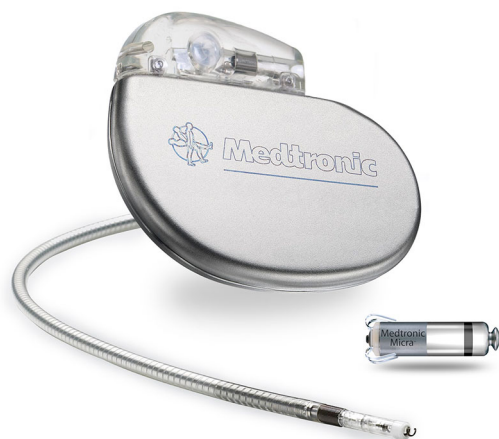
Fig. 6 Traditional pacemaker vs. Micra. Reproduced with permission of Medtronic, Inc
