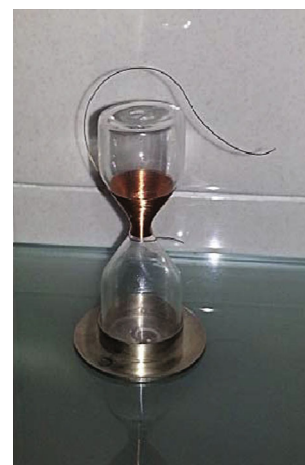
Fig. 5 The magnetic bottle with conical solenoid used in the experiments
