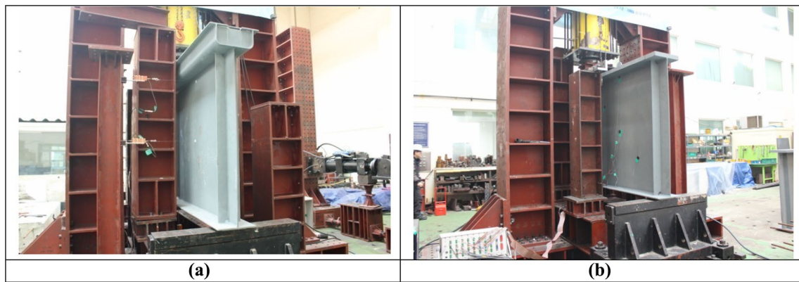
Fig. 4 Shear buckling tests of a proposed plate girder and b ordinary plate girder
