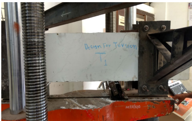
Fig. 3 Beam no. T1 after cracking
