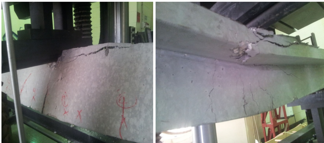
Fig. 7 Crack pattern and shape of triangular and T-beams after collapse
