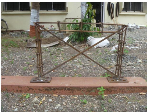
Fig. 2 Reinforcement details of frames
