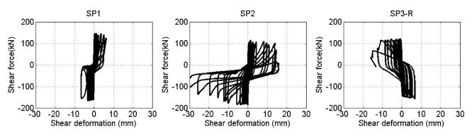
Fig. 19 Beam shear force-shear deformations relationships for SP1, SP2 and SP3-R specimens.
