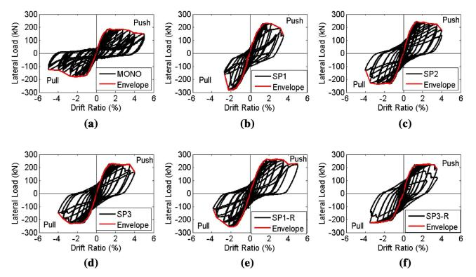
Fig. 16 Lateral load-drift ratio relationships for monolithic and precast connection specimens.
