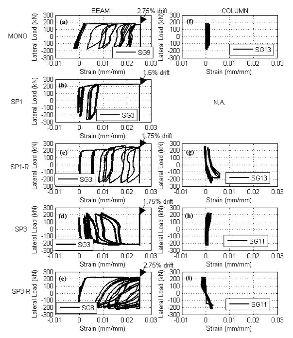
Fig. 18 Measured longitudinal bar strains of beams and columns of connection specimens.
