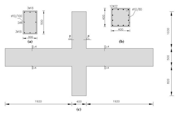
Fig. 4 Geometry and reinforcing details for monolithic specimen a beam section, b column section, and c interior connection.
