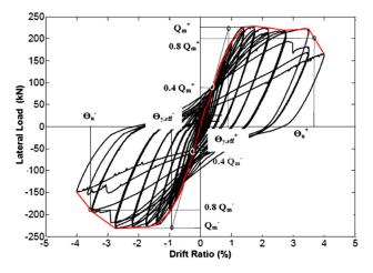
Fig. 20 Quantification of strength and ductility of test specimens.
