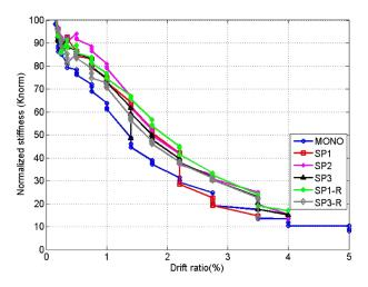
Fig. 23 Normalized secant stiffness (K<sub>sec</sub>) of test specimens for corresponding drift ratios.
