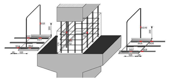
Fig. 13 Installation of strain gauges on beams and column reinforcing bars (units in mm).
