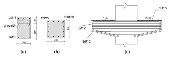
Fig. 8 Geometry and reinforcing details of precast specimens, a beam cross section, b column cross section, and c corbel details.
