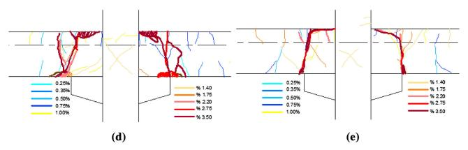
Fig. 14 Damage patterns of test specimens at each drift ratio and the end of test. a MONO, b SP1, c SP1-R, d SP3, and e SP3-R.
