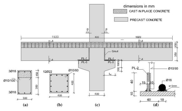
Fig. 5 a Beam, b column cross-sections, c front view and dimensions of the hybrid beam-column connections, and d welding detail of beam bottom longitudinal rebars to beam support plate (PL-1) and stirrups to vertical plates (PL-2) for SP1, SP2 and SP3 specimens.
