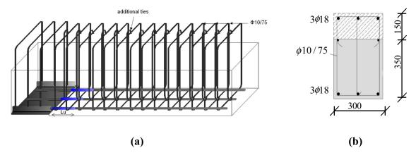
Fig. 9 a Application of unbounded length and b beam cross-section details of SP3-R specimen.
