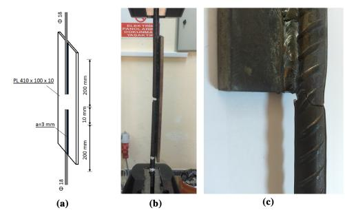
Fig. 2 a Schematic view of welded rebar-plate specimen, b specimen during tensile test, and c rupture of rebar with a clear necked region.
