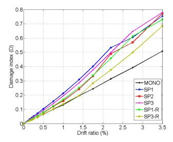
Fig. 25 Damage indices obtained for each test specimen.
