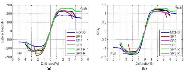
Fig. 21 a Lateral load-drift ratio envelopes of test specimens and b normalized envelopes of test specimens.
