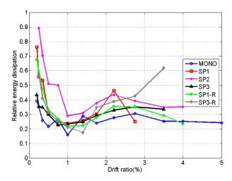
Fig. 24 Relative energy dissipation ratios  $(\beta_i)$  of test specimens.
