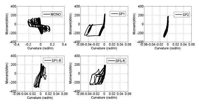
Fig. 17 Moment-curvature relationships of beam-column connection specimens.
