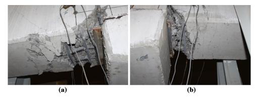
Fig. 15 a Initiation of rebar buckling at the left beam (Beam 1) and b the rupture of rebars at the right beam (Beam 2) for SP1 specimen at 2.2% top drift.
