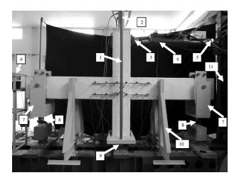
Fig. 10 Components in experimental set-up: (1) axial load frame, (2) hydraulic jack, (3) hinge, (4) actuator, (5) load cell, (6) reference frame, (7) pendulum support, (8) load cell, (9) fixed support, (10) out-of-plane support frame, (11) steel reaction frame.
