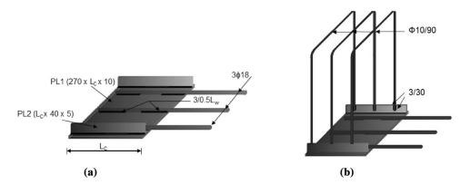
Fig. 6 a Perspective view of beam longitudinal rebars welded to beam support plate (PL-1) and b stirrups welded to additional vertical plates (2 × PL-2).
