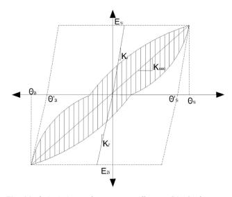
Fig. 22 Calculation of secant stiffness (K<sub>sec</sub>) for test specimens.
