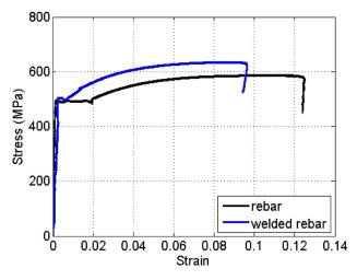
Fig. 3 Tensile test results for an 18 mm diameter single rebar and a rebar welded to plate.
