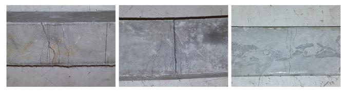
Fig. 4 Multiple-cracking behavior as seen in the failed specimen.
