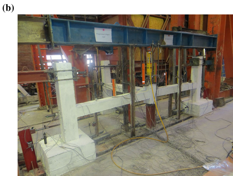
Fig. 5 Setup of the test specimens. a Test setup (in-plane frame). b Test setup (3D view).
