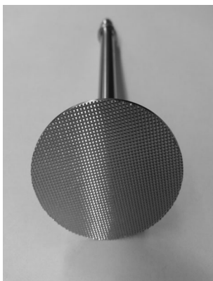
Fig. 1 Serrated bob plate used in the measurements to minimize the effects of slip and settling.
