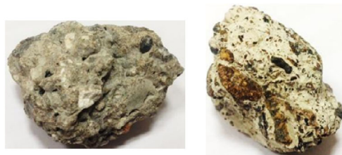
Small size aggregate connected by mortar
