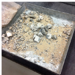
(d) Grade 4 - Mixture of coarse and fine aggregate along with impurities such as wood and plastic pieces
