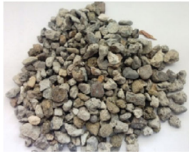
(b) Grade 2 - maximum size of 25mm
