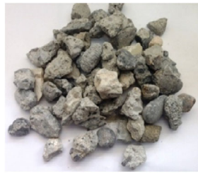
(a) Grade 1 - maximum size of 10mm
