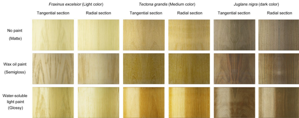
Fig. 2 Example of 18 difference kinds of wood original samples reconstructed in the 3D software. Including 3 kinds of wood colors (light, medium, and dark color), 2 kinds of grains (radial, tangential), and 3 kinds of glosses (matt, semigloss, and glossy). Each of them
