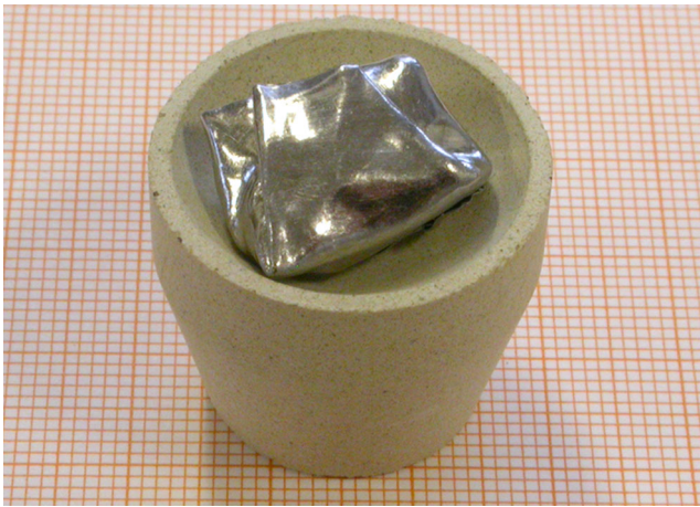
Fig. 1 Lead pouch containing the specimen and Ag, closed and placed on a cupel made of magnesium oxide, ready to undergo the in-furnace cupellation process
