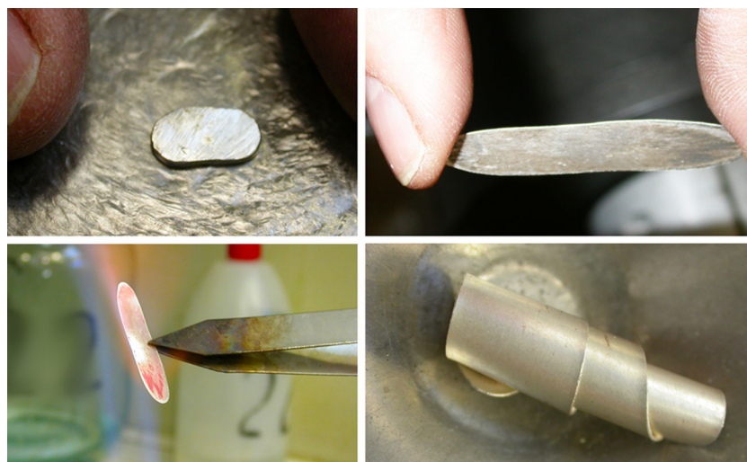
Fig. 14 The four stages of the cornet preparation are here represented. First the bead is hammered, flattened and rolled to a thin strip (top right), then flame annealed by means of a Bunsen apparatus and cornet shaped by hand
