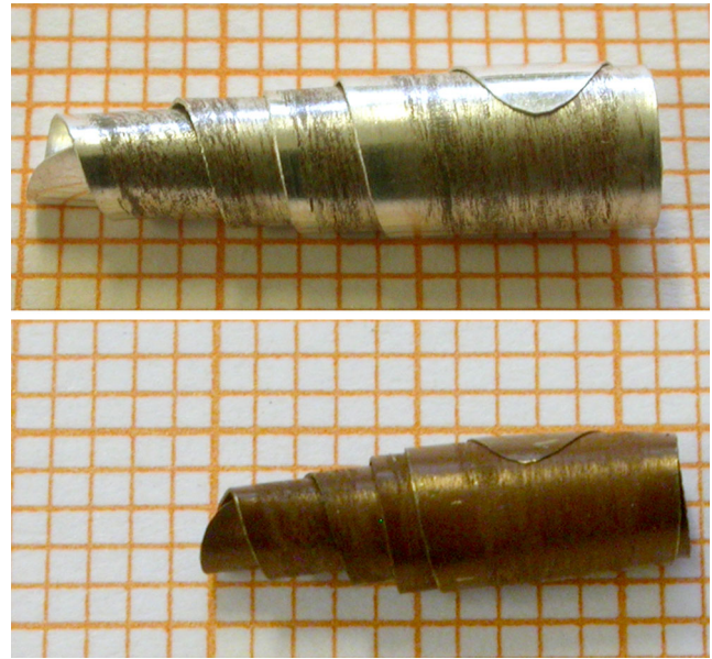
Fig. 21 The same cornet before and after partition is shown in the upper and lower part of the figure, respectively. See the size reduction that the cornet undergoes during the process. After partition, the cornet becomes typically brown, but preserves its initial shape
