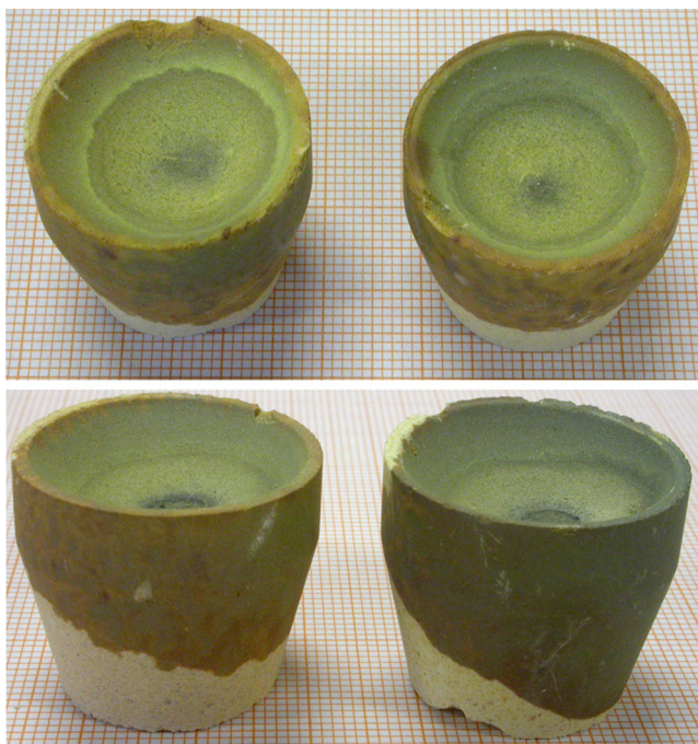
Fig. 5 Aspect of the cupel after the cupellation process. The greenish stain is due to the absorption of Pb and base metals oxides
