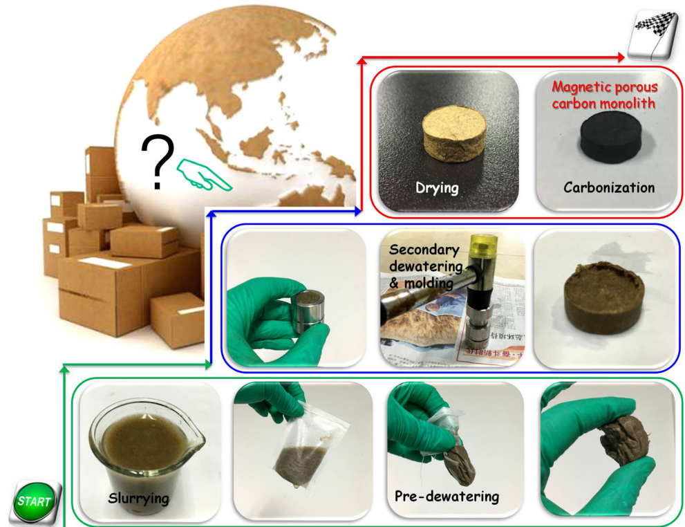
Fig. 1 Fabrication process of porous carbon monolith
