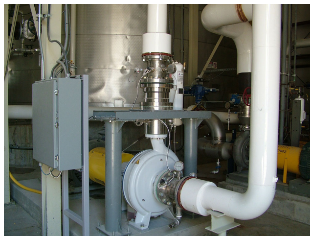
Fig. 2 Control flow cavitation unit sets up at commercial scale
