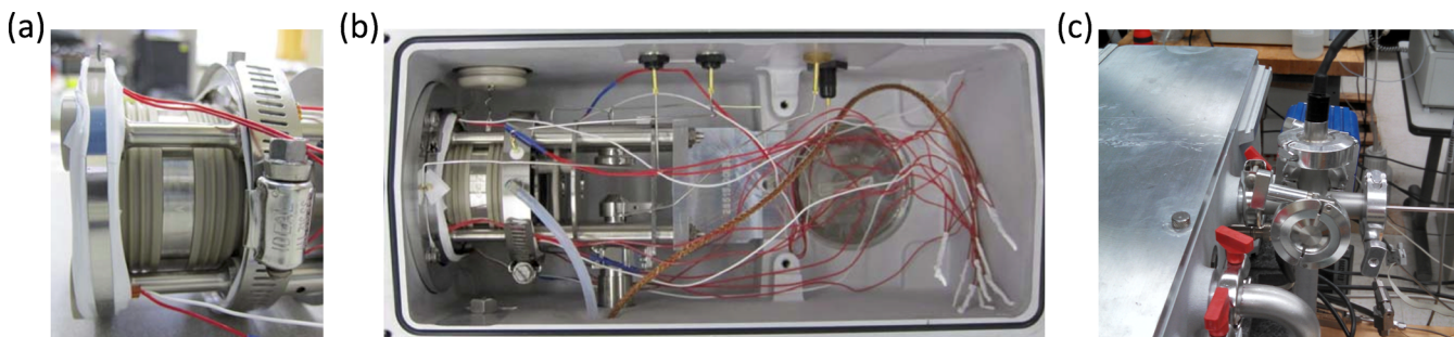
Figure 1. Modified Bruker Esquire ion trap: (a) ion trap with attached heating elements on end caps, (b) vacuum manifold, and (c) tee used for electrical and helium feed-throughs
