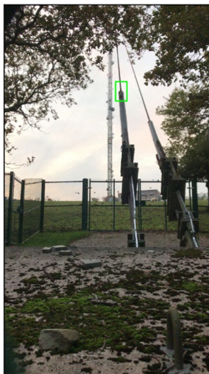
Fig. 8 A frame of high guyed mast cable anchor vibration and the template part (green rectangle)
