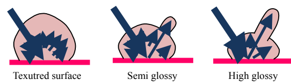
Fig. 3 Reflection from different type of surfaces.
