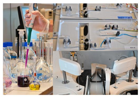
Three generations of analytical techniques: Hand-made permanganate consumption made to ensure the consistency of the long-term time series (*left*), auto-analyser (*upper right*), and a high-throughput discrete analyser (*lower right*). Photo by Jenny Svennås-Gullner (*left*) and Jens Fölster (*right*)
