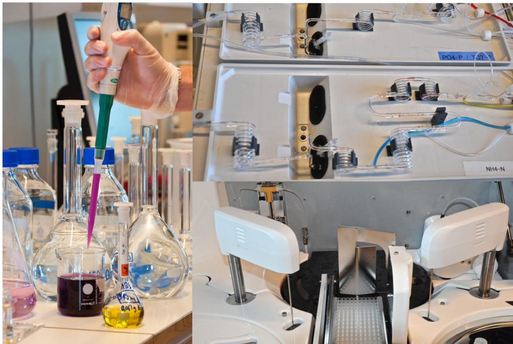
Three generations of analytical techniques: Hand-made permanganate consumption made to ensure the consistency of the long-term time series (left), auto-analyser (upper right), and a high-throughput discrete analyser (lower right). Photo by Jenny Sverrnäs-Gullner (left) and Jens Fölster (right)
