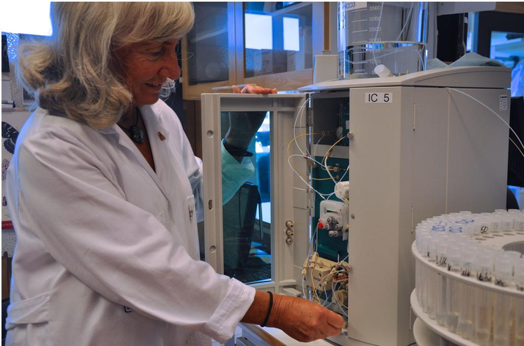
Gun Hölling who has worked with environmental monitoring since 1971 with the ion chromatograph, which replaced the old Macereth method for sulfate in 1984. Photo by Jens Fölster
