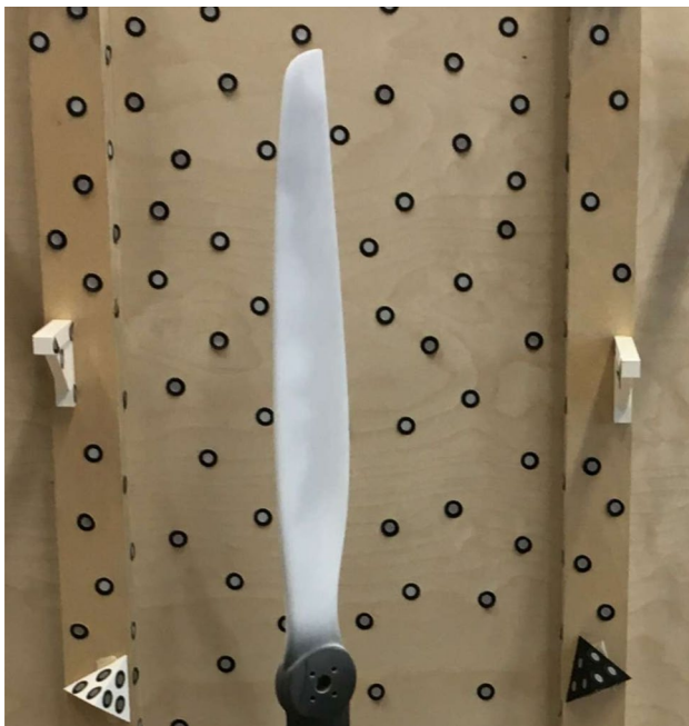
Fig. 3 Exemplary scan environment for a propeller with a diameter of 0.66m
