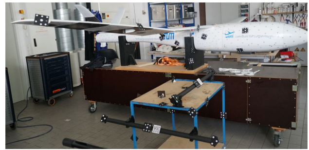
Fig. 2 Scan environment for large objects using the MaxSHOT 3D to capture the reference system [15]
