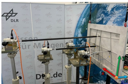
Fig. 13 Aluminum plate configuration for force and moment of force control
