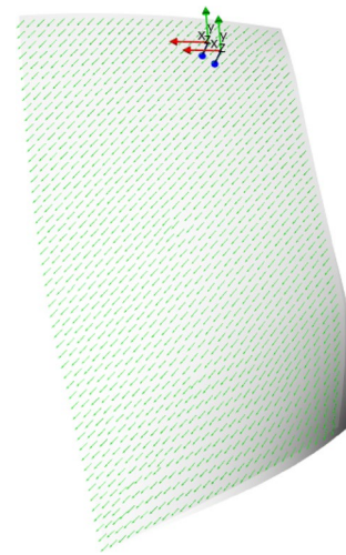
Fig. 7 ACP actuator model with actuation directions for the pressure side shown in green
