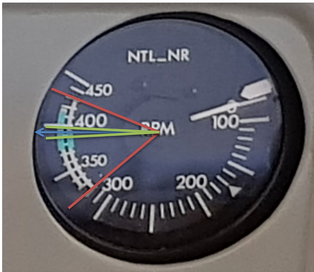
Fig. 6 N_r range limitations in flight (inner region, in green) and autorotation (outer region, in red)
