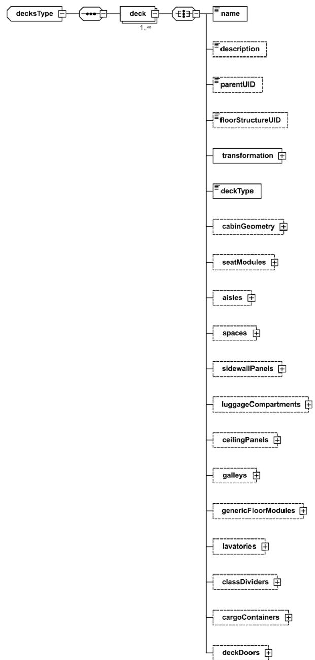
Fig. 7 XSD diagram of the deck node
