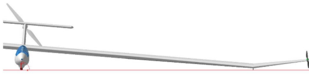
Fig. 23 Ground clearance analysis for icaré 2 wingtip propellers
