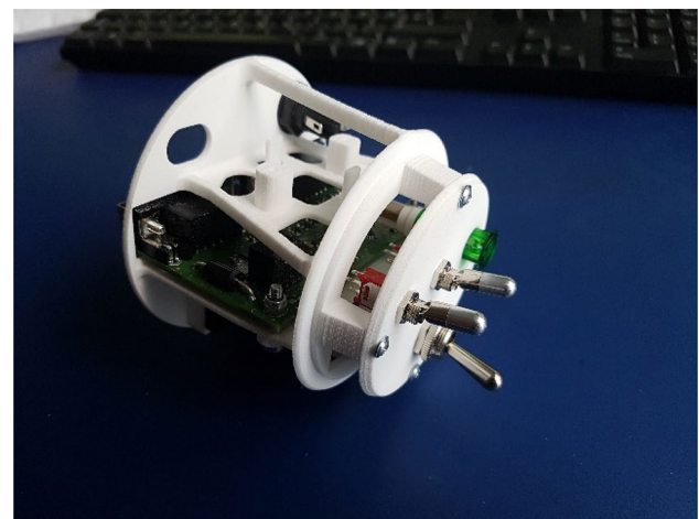
Fig. 26 Power distribution and control unit
