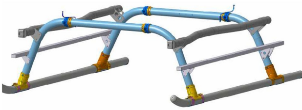
Fig. 7 Original, fully detailed CAD model of the EC135 landing gear
