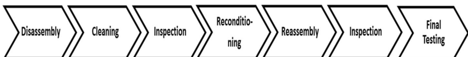
Fig. 1 A generic remanufacturing process chart based on the steps described in Steinhilper [53]
