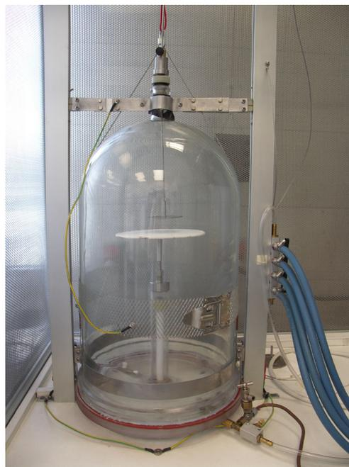
**Fig 1** Prototype generator of cold plasma
