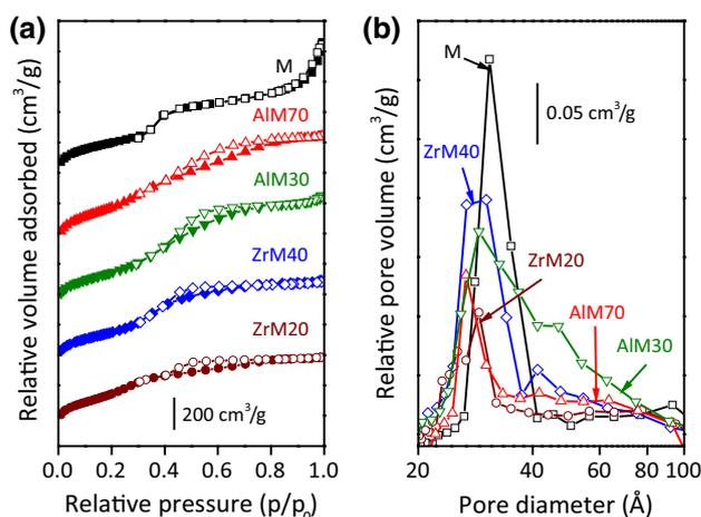
**Fig. 1** N<sub>2</sub> physisorption isotherms (a) and pore size distributions (b) of unmodified and modified mesoporous supports. Full and unfilled symbols represent the adsorption and desorption branches, respectively. The samples were degassed under vacuum and measured using a Micromeritics-ASAP 2010 automatic analyzer at liquid N<sub>2</sub> temperature
