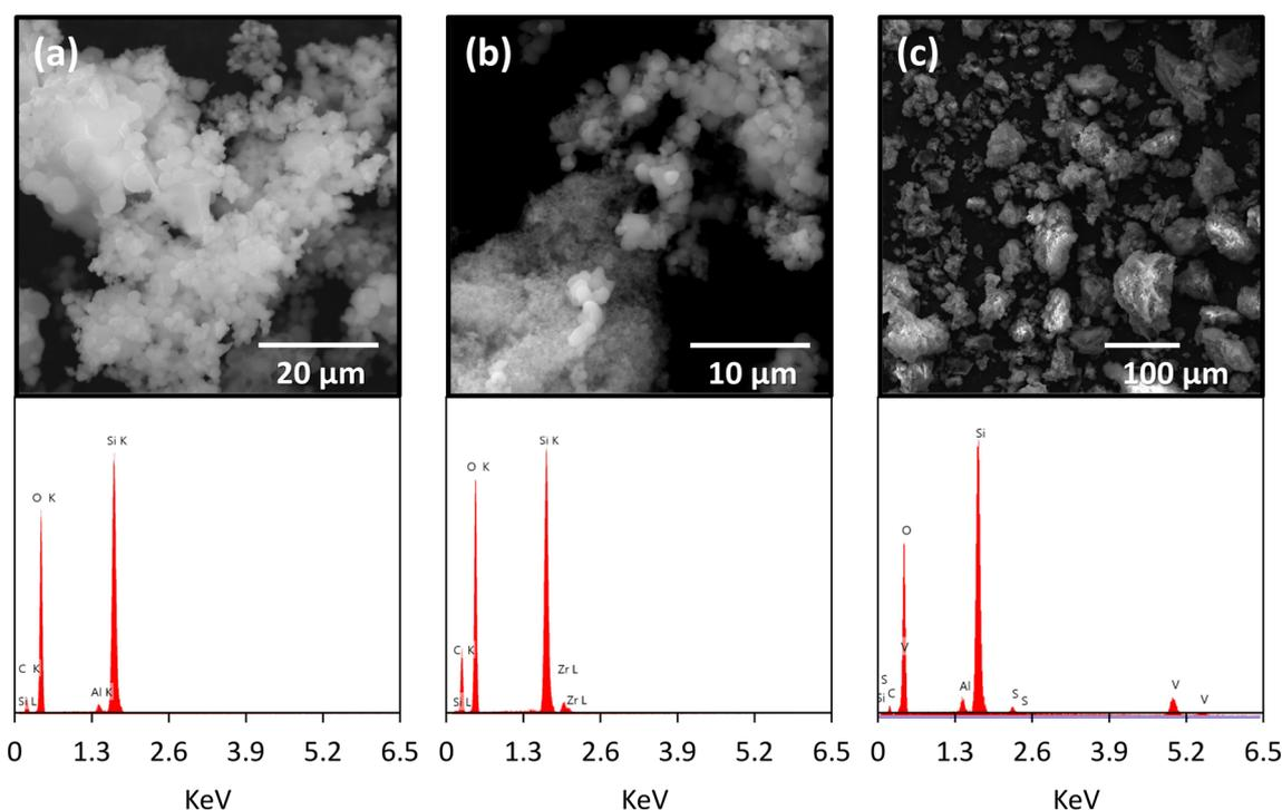
**Fig. 2** SEM (top) micrographs and elemental analysis spectra (EDX, bottom) of the ZrM40 (a) and AIM30 (b) supports and sulfided VAIM30 catalyst (c). The analyses were carried out using a FEI Quanta 250 SE microscope coupled to an EDAX model Octane SDD analyzer
