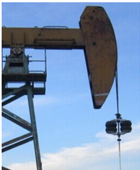
Fig. 2 Shock absorber with pneumatic spring (Lu 2015)
