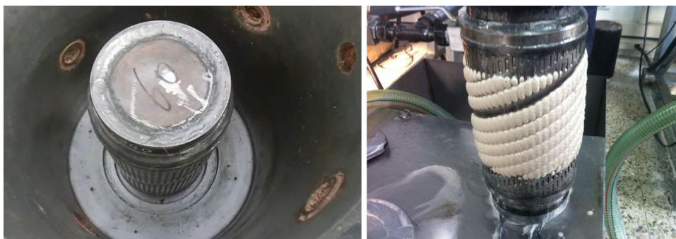
Fig. 3 Screen contrasted before and after the experiment under different water content
