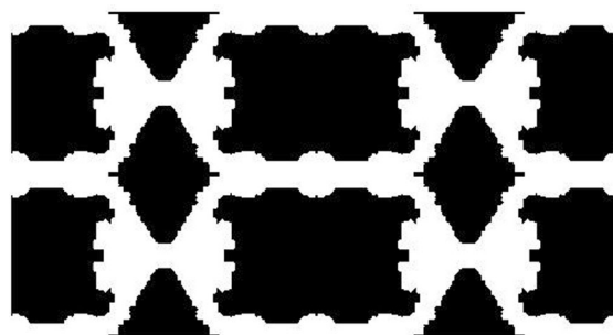
Fig. 8 Simplified pore structure, 264 \times 502 \text{ lu}^2 , 38 % porosity
