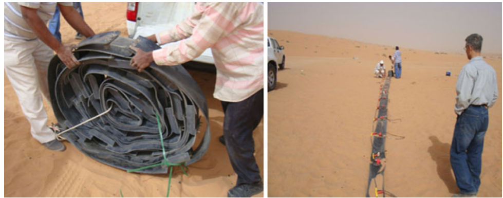
Fig. 5 Field photographs and the layout of the streamer
