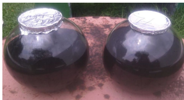
Fig. 2 Solar irradiation of textile wastewater samples in the presence of \text{Fe}_2\text{O}_3 NPs for irrigating on plants
