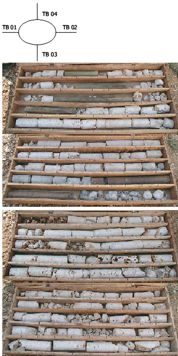
Fig. 3 Borehole orientation at the barrage site and cores from TB03 (floor) and TB04 (roof) in comparison
