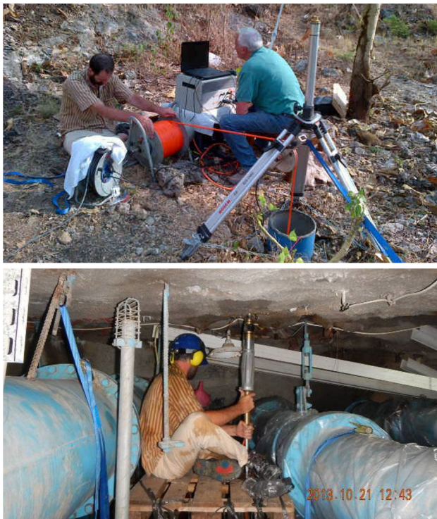
Fig. 9 Borehole camera in use on ground surface and at the cave roof
