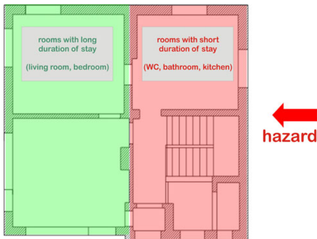
Fig. 1 Distribution of the different rooms according to occupancy time and hazard potential (Holub and Hübl 2008)
