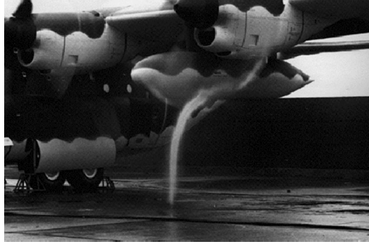
Fig. 1 Occurrence of a ground vortex on the outboard propeller of aircraft C130 (Campbell and Chambers 1994) (reprinted with permission from J. F. Campbell and J. R. Chambers, “Patterns in the sky: Natural visualization of aircraft flow fields,” NASA Report No. SP-514, 1994. Used with permission of NASA)
