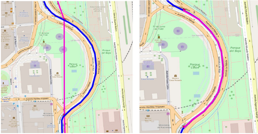
Fig. 11 Left: Bus line #152, static route (blue), real time data points (red), generated route (pink); Right: Trajectory corrected with the map-matching algorithm
