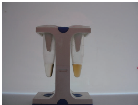
Figure 3 Magnetic separation of MNPs (left) and MNP/MWNT nanocomplex (right). Both can be easily magnetically separated under the external magnet (between the two tubes). As shown in the figure, however, the MNP/MWNT nanocomplex is more rapidly separated (within 30 s) while MNPs are not separated within this short period. This is possibly because the particle sizes of the nanocomplex are significantly larger
