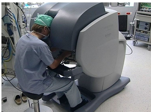
Fig. 5 The DaVinci operation robot (first generation): surgeon's console (Da Vinci first Generation, Intuitive Surgical, Intl.)
