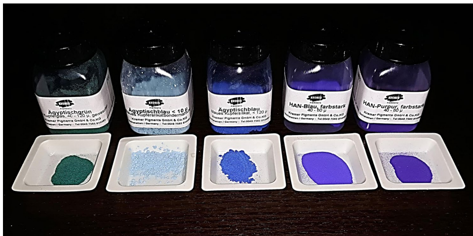
Fig. 8 Image of modern EB and related pigments marketed by Kremer Pigmente. From the left: 10,064 Egyptian green, 100,601 Egyptian blue (particles < 10 \mu\text{m} ), 10,060 Egyptian blue (particles < 120 \mu\text{m} ), 10,072 Han blue (i.e., CB) and 10,075 Han purple (i.e., CP) (colour figure online). Adapted from Nicola (2019)
