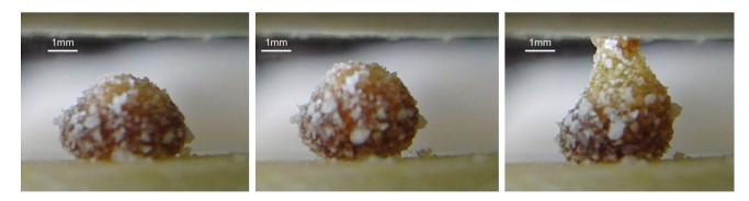
Fig. 6 The sequence of images illustrating the behavior of a 20  $\mu$ L crude petroleum oil marble exposed to an electric field; the left image depicts the initial state of the marble and the right shows the marble exposed to the electric field of  $E \simeq 10^6 \frac{V}{m}$
