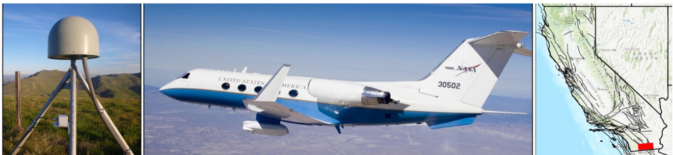
Fig. 1 Instruments and data products. Left: GNSS station. Middle: UAVSAR pod is attached under the aircraft. The instrument looks left at an angle of 27–63° to the ground. Right: California showing faults in black and location of the displayed UAVSAR swath in Fig. 2 in red
