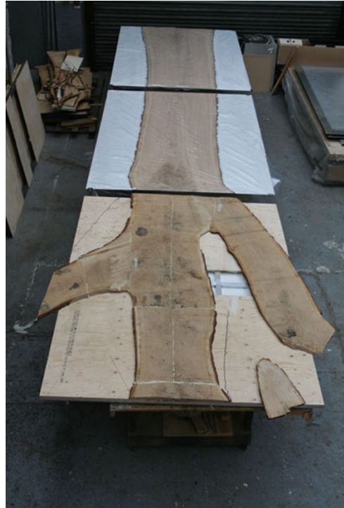
Ceiling sections being prepared at the fabricator’s studio. Kiln-dried planks bonded to aluminium honeycomb sheets routed to 3-mm-thin veneers (©Mike Smith Studio)
